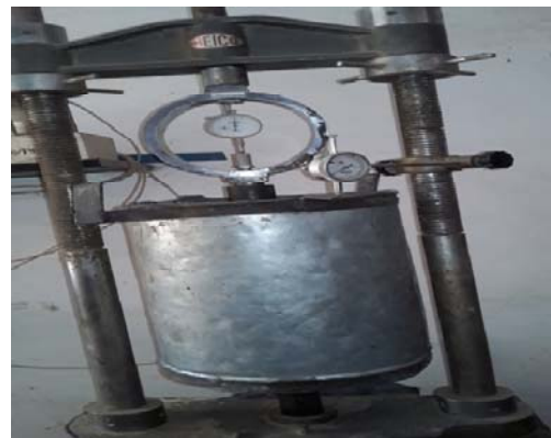
Figure 2: Schematic Picture of Model Testing Tank under Loading Frame.
