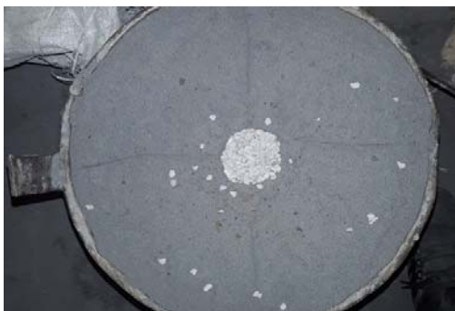
Figure 1: Schematic picture of stone column embedded in pond ash bed.
